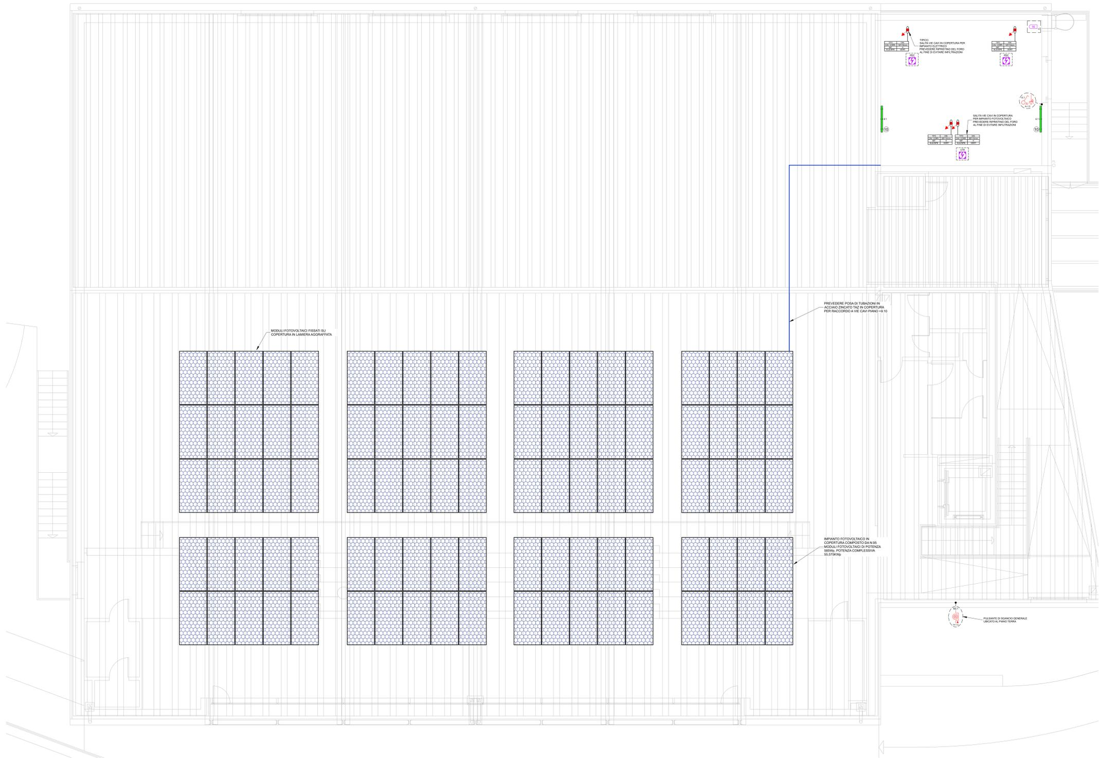
MODULI FOTOVOLTAICI FISSATI SU COPERTURA IN LAMIERA ADGRUPPATA
